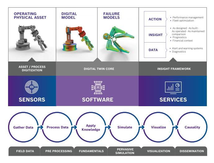
The modern Digital Twins are dynamic software models of assets or processes that enable real-time monitoring and improve process efficiencies. It improves enterprise decision-making by providing information on maintenance and reliability, insights into how an industrial asset, system or product could perform more effectively, data about new productions, and information on drivers of efficiency.
